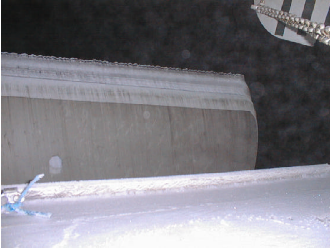
Figure 5. 12 cm of ice on tip.
