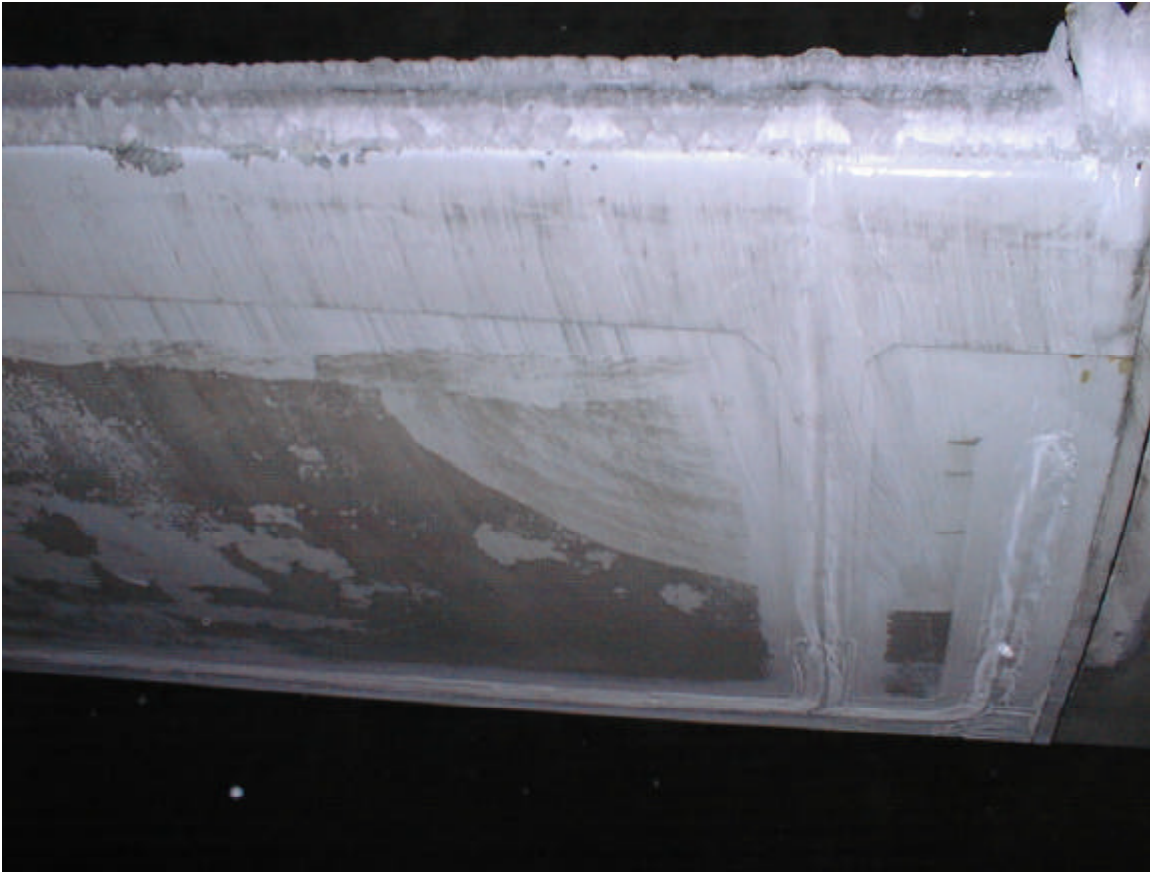
Figure 2. Two peaked ice on leading edge
